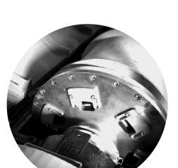
The Mammoth-2276 larger bowl is complemented by a KHT-125 96:1 gearbox. This gearbox creates an output of 175,000 in/lb—far superior to the industry average which typically only creates 30,000 to 53,000 in/lb. Ultimately, the KHT-125 gearbox facilitates an increase in the volume of solids that the Mammoth-2276 can remove. This is critical when working with weighted fluids where the required volume of solids to be removed is substantial, requiring additional torque from the centrifuge.
