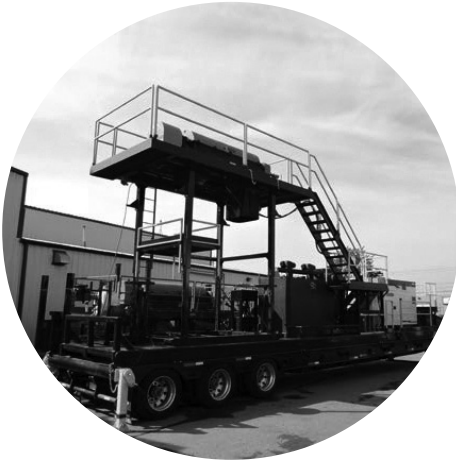
Kayden Mammoth-2276 Centrifuge, Polymer tank and 150kva diesel operated generator, mounted on triple tandem wheeled trailer.
