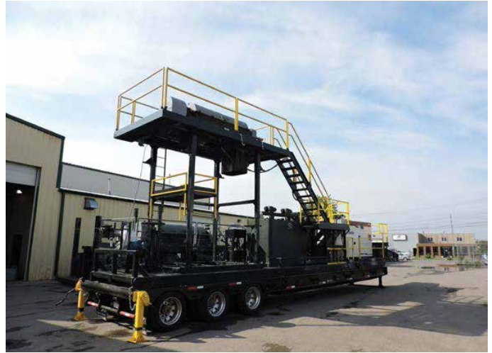
Kayden Mammoth 2276 Centrifuge and Dewatering System, equipped with 150kva diesel operated generator; mounted on triple tandem wheeled trailer.
